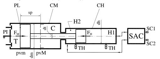
Figure 2. The functioning scheme of the monoregime thermo-hydraulic generator
